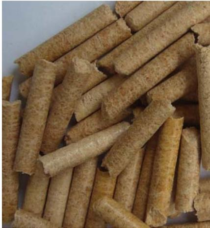
The saw dust will go through a pelletization process which includes crushing, drying, pelletizing, cooling and packing in order to form a quality saw dust pellet product.
