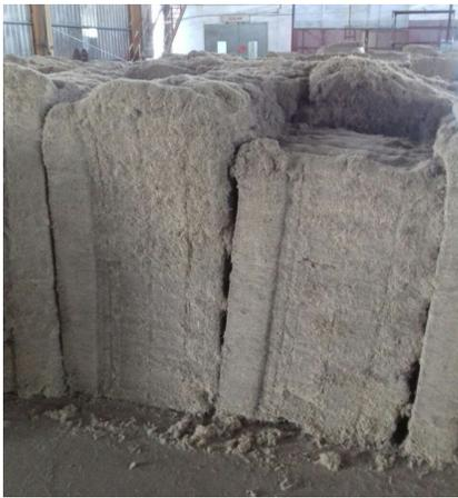
The short dry palm fibre from Biofuel Resource is collected from the palm fibre sieving process. We are segregating **long palm fibre** and **short palm fibre** during our process. The long fibre will be bundle and export for mattress application. The *short palm fibre* will gather and send for *biomass application*.
